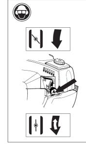
position. The start throttle position is obtained by setting the choke control in the choke position and then returning it to its original position.
